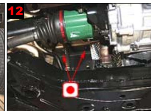
12 Cross member behind engine: Remove 2 clips and treat via holes.
