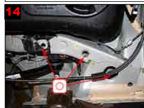
14 Longitudinal member/rear section before rear wheel casing: Treat via existing holes.
