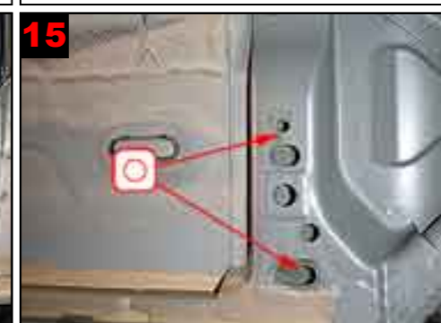
15 Small cross member after front wheel arch: Treat via existing holes
