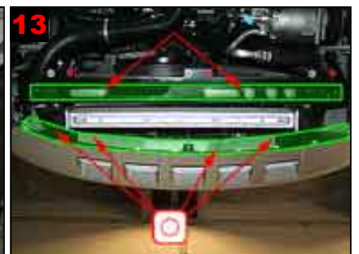
13 Treatment of cross member under radiator and bumper via existing holes.
