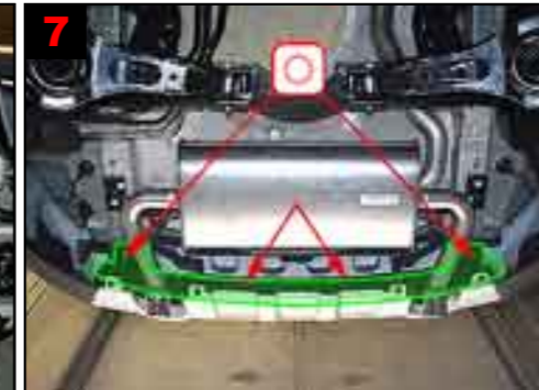
7 Rear panel: Treat between front wing and rear panel and treat U-member for bumper. Reinforcements: Treat via existing holes.
