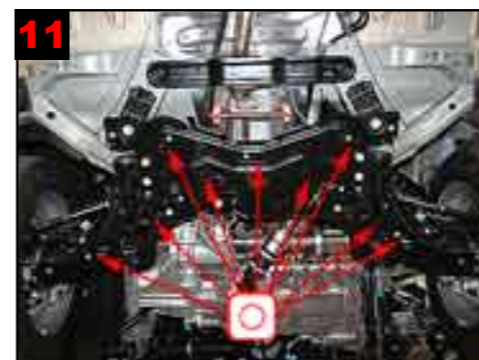
11 Front axle assembly/supports: Treat via existing holes and gaps.
